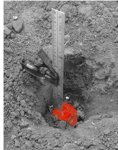
Ensure that the metal-detector Test areas are metal free before the target mine is placed and that target mines are placed at the required depth. The detector Test area is often positioned alongside the detector Calibration area but need not be. Both areas must be clearly marked.
