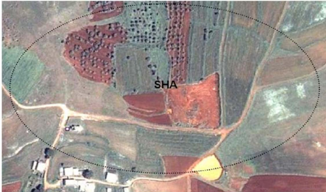
Figure 1 – The picture illustrates a possible SHA generated during an impact survey or other claim of presence of hazard.
